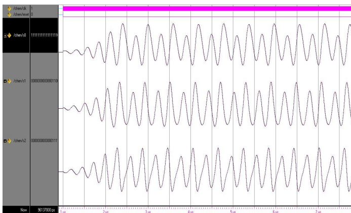
Fig. 17. ModelSim simulation results of the chaotic signals x , y and z .
